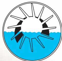
Liquid level when pump is at rest.
